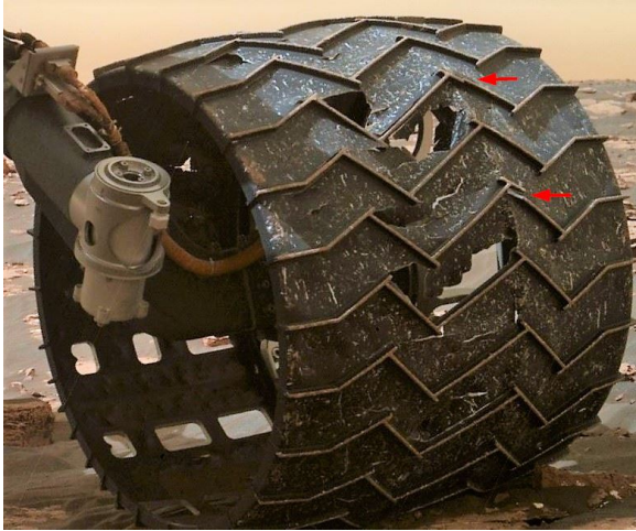
Figure 1: Damage shown on Curiosity rover wheels due to small rocks. [3]
